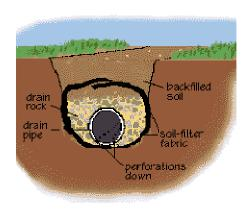
Alternatively, you can bury a length of perforated plastic drainage pipe that leads water away from the downspout and into a disbursing field. Or you can, as illustrated, combine the two. It's the same principle, and almost as much work. ❖
